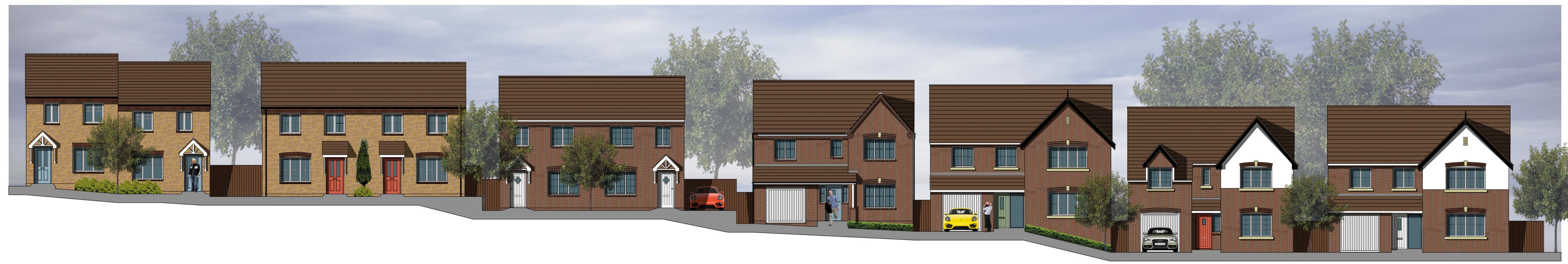
Street Scene 4 Plot 73 SO2+ (109.30 FFL) Plot 72 SO2+ (108.85 FFL) Plot 71 SO3 (108.70 FFL) Plot 70 SO3 (108.70 FFL) Plot 34 Cherry (107.90 FFL) Plot 33 Cherry (107.90 FFL) Plot 32 Maple (107.15 FFL) Plot 31 Alder (106.70 FFL) Plot 30 Acacia (105.50 FFL) Plot 29 Alder (105.50 FFL)
